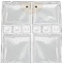
Figure 4-4: Seal with the loading well
